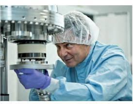
With the SPM 150 Aarhus (STM & NC-AFM), SPECS offers an instrument of unique stability and productivity for surface studies with atomic resolution. Atomic growth and catalytic processes on surfaces can be equally observed at different temperatures. A second example for a state-ofthe-art surface microscope is the Low Energy
