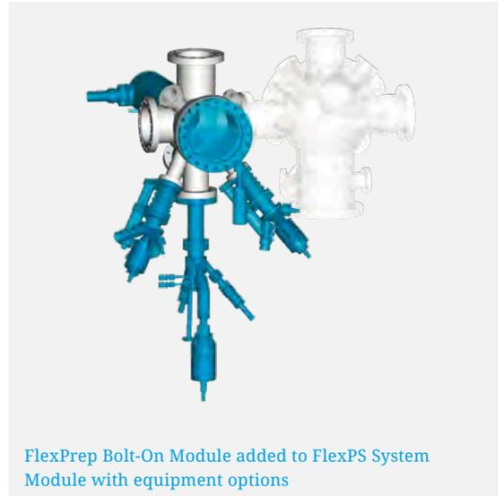
FlexPrep Bolt-On Module added to FlexPS System Module with equipment options
