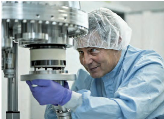
SPECS specialist assembles a high voltage 2D-CCD detector to a PHOIBOS 150 HV
